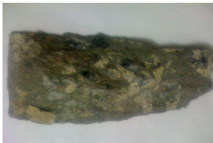
Fig 5: Failure plane of concrete under compression
